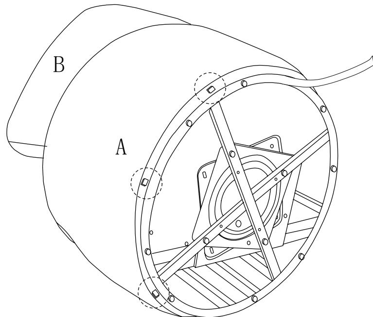
Before assembly, please remove the small wooden blocks and the non-woven fabric on the tube.
